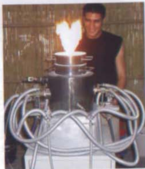
Angelo Themelis heat treating geuda using the Sri Lankan Lakmini gas combustion furnace.
