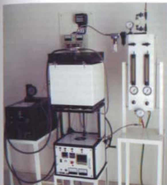
Fig. 10-63. Gemlab model 181 1800°C vertical muffle, bottom loading electric resistance furnace fabricated by the author and available commercially. The furnace system consists of a) the furnace module, b) power module, and c) atmosphere control module. The furnace operates from any 208/240 Vac @ 50 Hz, 15 Amp single-phase electric outlet Capacity 3000 ct of ruby-sapphire per load. Los Angeles, CA. 2003.
