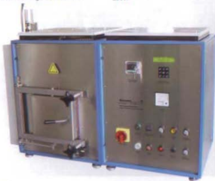
Fig. 10-63. Gemlab model 181 1800°C vertical muffle, bottom loading electric resistance furnace fabricated by the author and available commercially. The furnace system consists of a) the furnace module, b) power module, and c) atmosphere control module. The furnace operates from any 208/240 Vac @ 50 Hz, 15 Amp single-phase electric outlet Capacity 3000 ct of ruby-sapphire per load. Los Angeles, CA. 2003.
