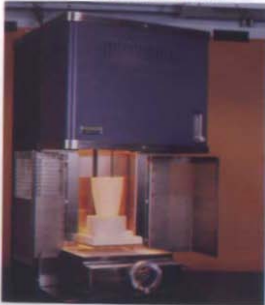
Fig. 10-60. Bottom-loaded electric resistance 1700°C box furnace by Linberg Co. Houston, TX., 1996.
