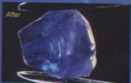
Sapphire before (top) and after (bottom) heated at 1650°C in air without chemical additives.
