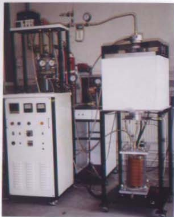
Fig. 10-60. Bottom-loaded electric resistance 1700°C box furnace by Linberg Co. Houston, TX., 1996.
